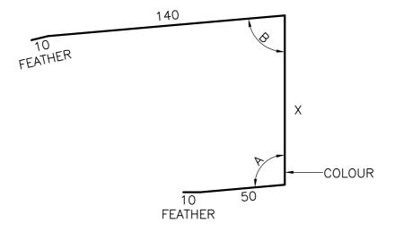
A - TO SUIT ROOF PITCH (90° + ROOF PITCH)
