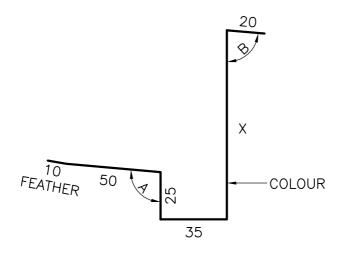
A - TO SUIT ROOF PITCH  $(90^{\circ} + ROOF PITCH)$
