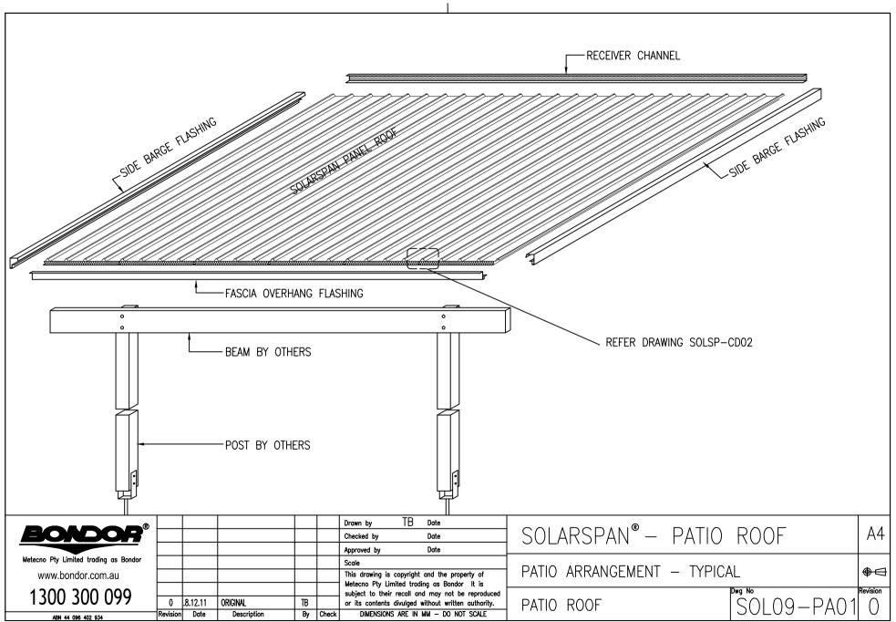
REFER TO SOLARSPAN WEBSITE www.soloarspan.com.au FOR LATEST VERSION OF THIS DRAWING.
